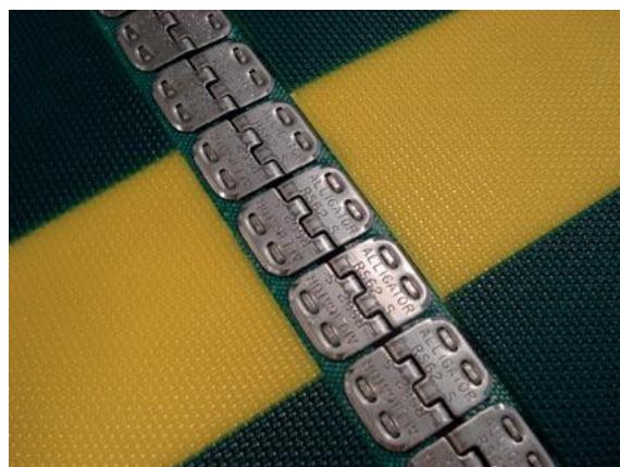
Detail of the Aster 22AF-Ski spliced with fasteners.
