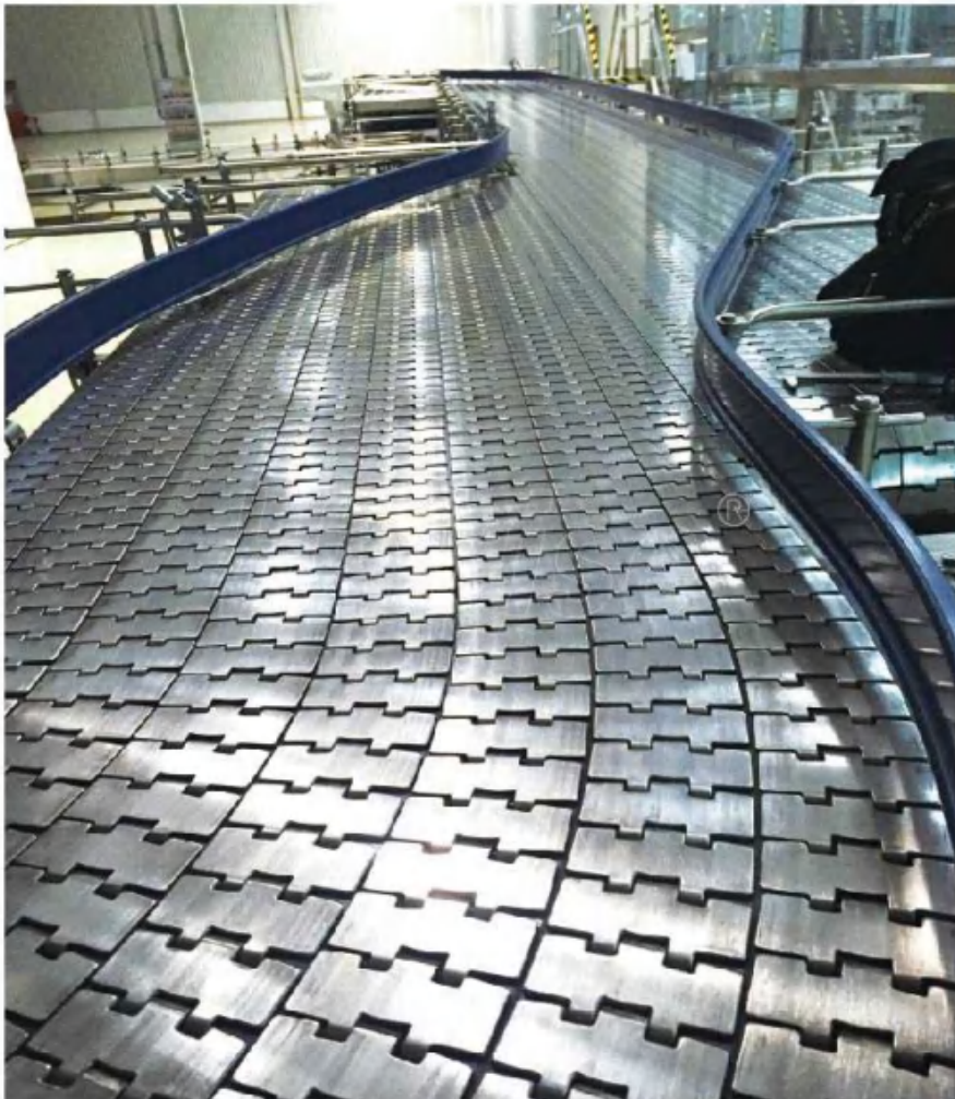
Metal Chain Conveyor Pretty Popular in Glass Bottle Industry
